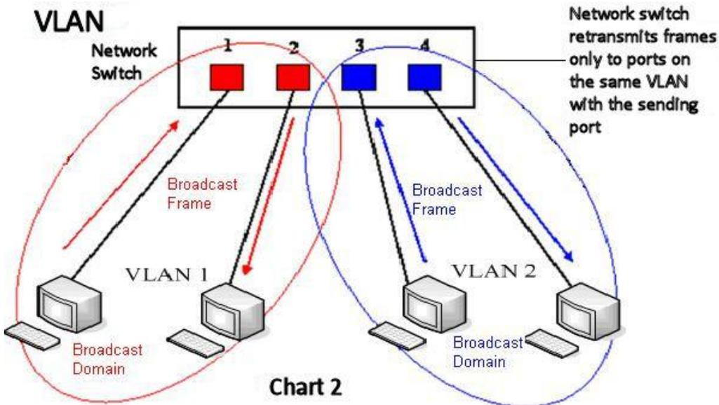
Chart 2 shows an example with two VLANs indicated by red and blue. In this example, frames broadcast from Port 1 will only go to Port 2 since Ports 3 and 4 are in a different VLAN. VLANs can be used to divide a network by restricting the transmission of broadcast frames.
